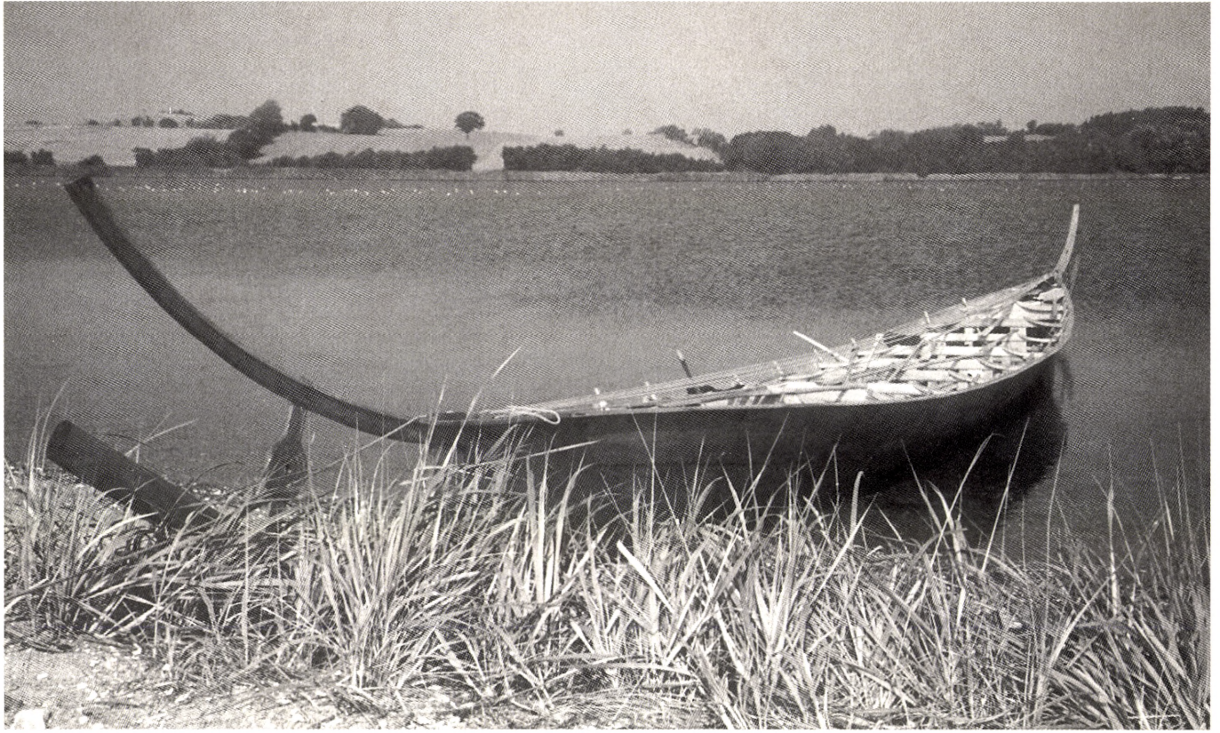
Plate 38. The Hjortspring boat. Recent trials have brought the boat above eight knots; dry rides in waves of one and a half metre in open sea are also possible. (Photo: Klavs Randsborg).
